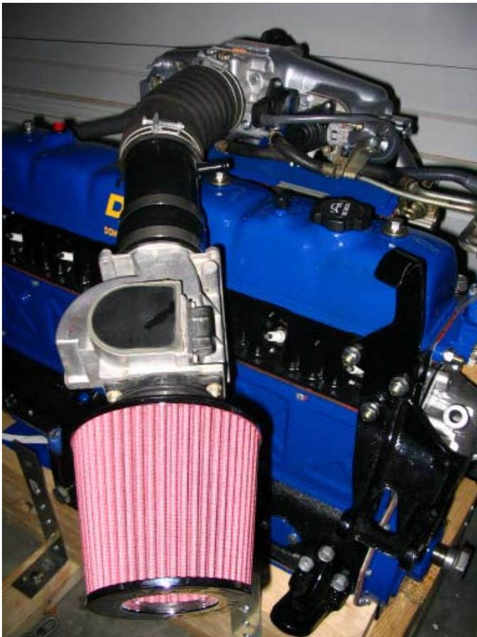
Figure 6. Intake from cone filter to AFM.
