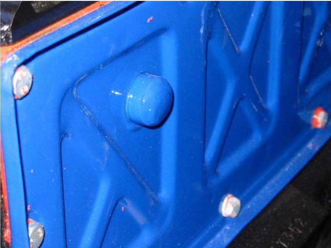
Figure 4. Plugged PCV port on 2F side cover.
